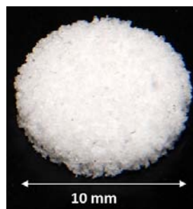
Figure 3-1: Representative photograph image of 10 mm diameter, 2 mm thickness PDMS scaffold of 250 to 425 \mu\text{m} pore size.
